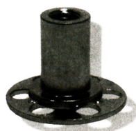
316 Stainless Steel female threaded insert on a blind 23mm diameter base plate
