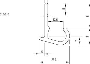
TILA continuous hinge drawings shown in the scale of 1:1
