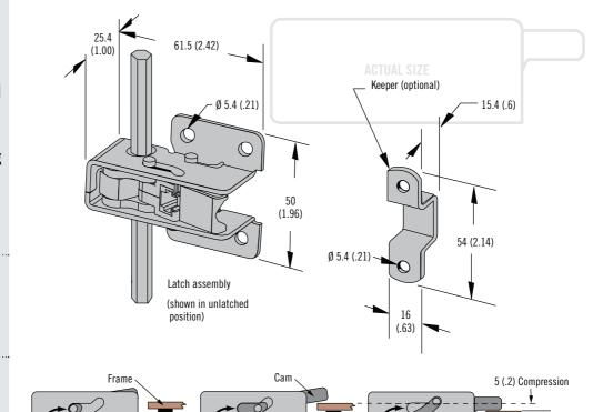
\* Measure your **Grip** from the latch mounting surface to the inside frame surface, with gasket compressed
