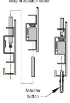
Mount keeper with M5 (No. 10) screws. Keeper can be adjusted 3.2 (.13) from center both vertically and horizontally for proper alignment with latch.
