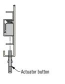
Remote Latching Style Insert extension rod and actuator button into brackets
