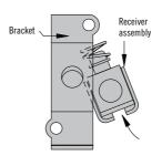
Insert extension rod into brackets, then slide receiver assembly into side of lower bracket and snap-in actuator button.
