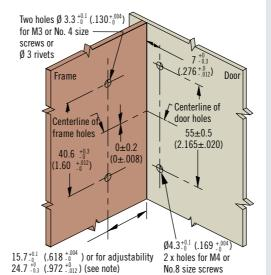
Note: These holes and dimensions are used only if adjustability through the use of slotted holes in catch is desired.
