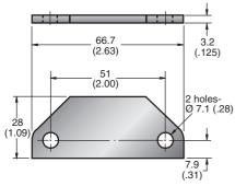
One supplied with each assembly. For extra shims order part no. *A2-54-501-11*.
