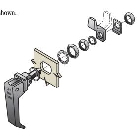
3. Pawl should be adjusted to GRIP measurement with the door open and the handle in the LATCHED position. Use two wrenches to tighten.
