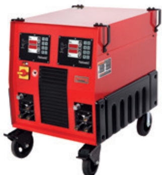
NELWELD 6000 Heavy duty drawn arc welder Welding current 300-2500 A step less Welding capacity at Ø 25 mm 10 studs / min. Through deck stud welding up to Ø 22 mm
