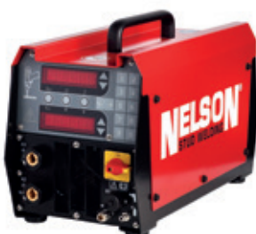
NELWELD 800i Mobile inverter based drawn arc welder Welding current 50-850 A step less Welding capacity Ø 3 mm to Ø 12 mm
