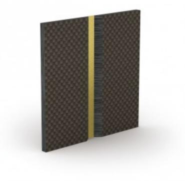
Hinge is constructed of rigid leaves and a flex unit. The rigid leaves are a glass fibre carbon hybrid. The Kevlar flex units are impregnated with a flexible urethane. Design for bond or screws assembly. No metallic component. Ultra light, ultra thin.
