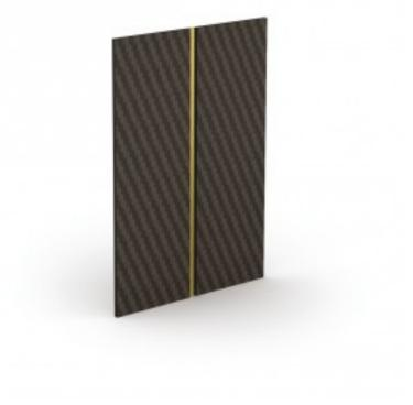
Hinge is constructed of rigid leaves and a flex unit. The rigid leaves are wowen carbon fibre in an epoxy matrix. The Kevlar flex units are impregnated with a flexible urethane. Design for bonding. No metallic component. Ultra light, ultra thin.
