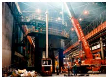
The world's largest bolt-style Superbolt being installed in a two-post hydraulic forging press.
