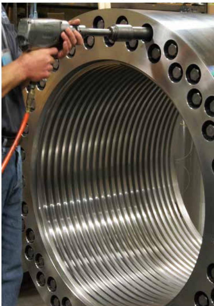
Assembling an enormous 1016 mm (40 inch) thread tensioner, used on a 50,000 ton press.
