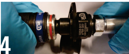
4 Check the red line is not visible – if red line is visible the connection is not safe to use
