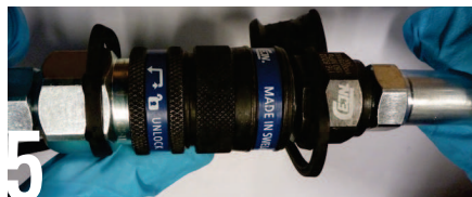
5 To close the safety locking sleeve (SLS) push the shroud forward to the back of the collar and rotate – release to lock
