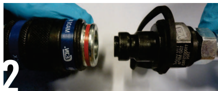
2 Insert the nipple into the coupling whilst the shroud is in the retract position
