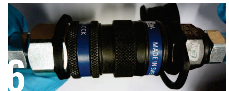
6 This image shows the SLS in the locked position – this joint is now safe to use
