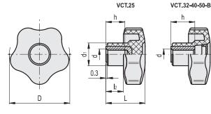
Code Description D d6H L d1 12 h 52 25 19 10 150534 VCT.25 AE-VO B-M5 M5 13 8 6 150544 VCT.32 AE-V0 B-M6 32 M6 23 15 10 12 11 150564 VCT.40 AE-VO B-M8 40 M8 27 17 12 18 24 150584 VCT.50 AE-V0 B-M10 50 M10 32 19 14 26 34
