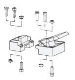
Prior to installation remove the slam latch cover as shown in the sketch. Socket head cap screws DIN 912, hexagon head screws DIN 933 and hexagon nuts ISO 4032 each with thread size M 6 can be used for mounting the slam latch.
