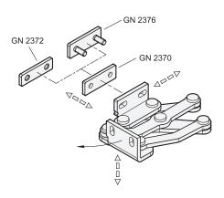
The Stainless Steel-Multiple-joint hinges can be adjusted in three planes during installation. For example, this allows tolerances to be adjusted or the required compressive forces for seals to be established. Two planes can be adjusted via the parallel or perpendicular slots in the fixing angle pieces. In the third plane, position corrections can be made using the Stainless Steel-Spacer plates GN 2370 (see page).
