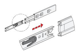
Type F has additionally a detach function through which the extension slides can be completely separated from one another in the area of the middle and inner slide. This feature not only facilitates mounting. It also allows the extension to be quickly removed, for example, when frequent maintenance work is performed on the components located behind.
