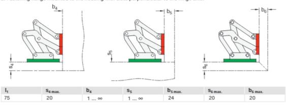
The design variants shown represent standard installation conditions. If the installation position of the hinge is changed or one of the two wall thickness dimensions is lower than s or b, the maximum achievable dimensions change independently of each other. This makes it possible in some cases to work with larger wall thickness dimensions than those specified with the same hinge size. A simple design check via CAD or a test setup is therefore recommended.
