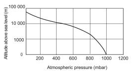
Comparison between atmospheric pressure values measured at sea level with the same values measured at different altitudes.
