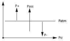
Pressure dimensionally represents a force per unit of surface, its unit of measurement is the Pascal (Pa symbol) which represents the pressure obtained when a force of 1 N (Newton) is exerted on the unit surface of  $1 \text{ m}^2$ . Therefore, the result is:
