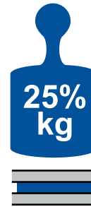
Horizontally mounted = 25% quoted load rating
